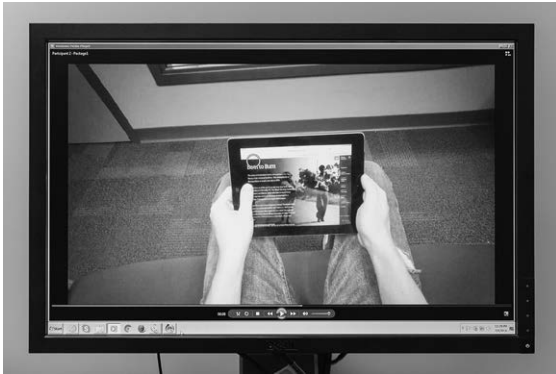
Photo by Nico Ciani. While participants interacted with longform journalism on iPads, researchers watched where the participants focused their attention, indicated by a red ring on the researchers' screen.
